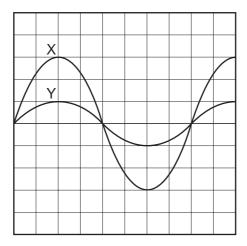
Signal X has a frequency of 50 Hz and peak voltage of 12 V.
