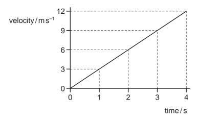
What is the displacement during the last 2 seconds of the motion?
