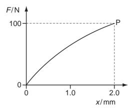
What could be the value of the strain energy stored in the wire when it is stretched to point P?
