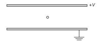
A small charged liquid drop, midway between the plates, is held in equilibrium by the combination of its weight and the electric force acting on it.
